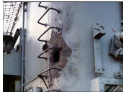
Rocket damage to HMS Antrim
