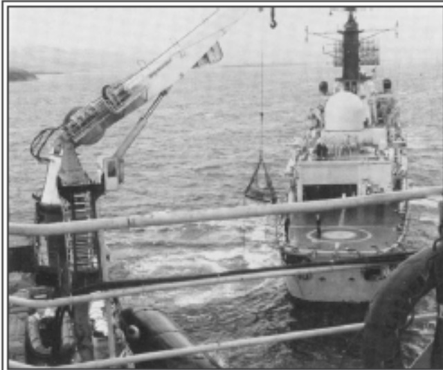
Figure 6: HMS Exeter being serviced by Stena Seaspread: the 100 ton crane in use. Note air filled Dunlop fender
