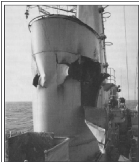
Figure 4: HMS Plymouth's funnel damage by 'something' that hit her during the action on 8th June
